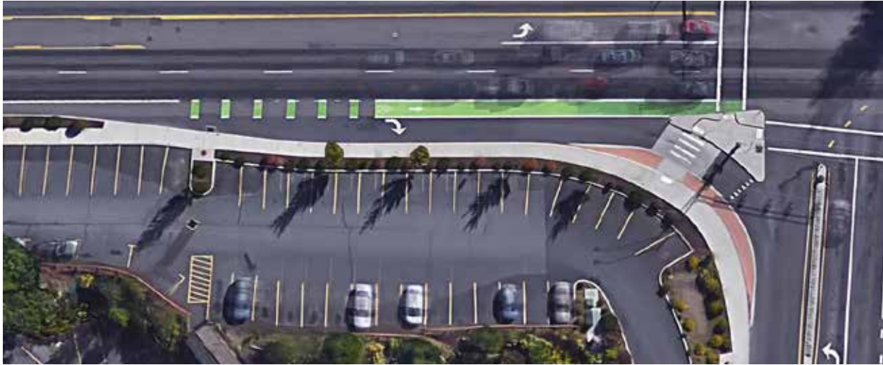
This example uses a raise, mountable apron at the corner to define a tight corner radius for passenger cars.
