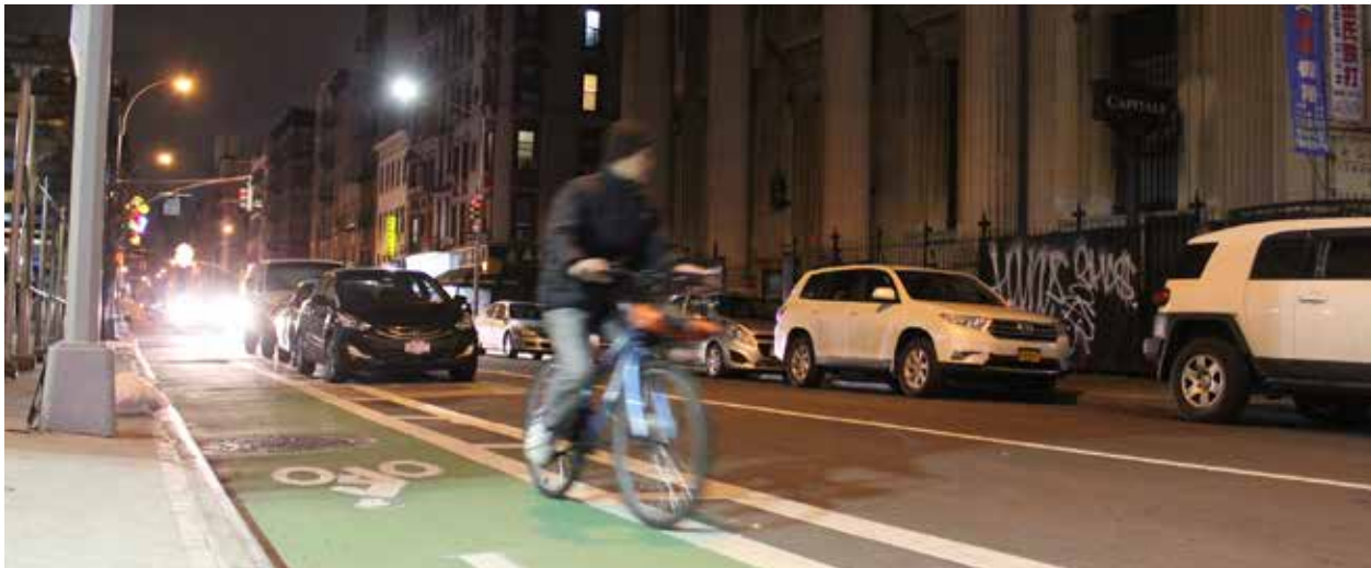
Street Level Separated Bicycle Lanes can be separated from the street with parking, planters, bollards, or other design elements.
