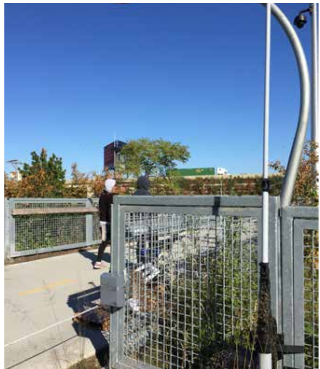
Figure 22. Example of an infrared sensor to count pedestrian and bicycle trips on a trail.
