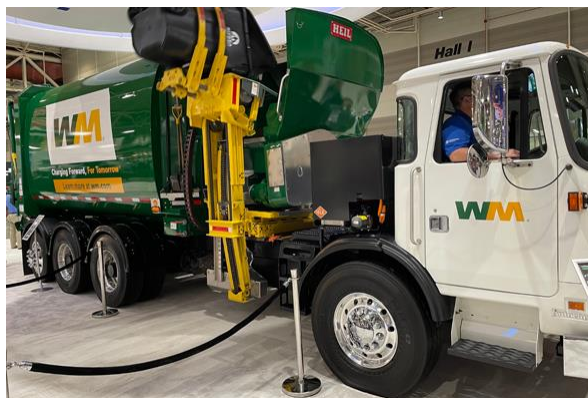
WM is piloting this fully integrated electric Class 8 collection truck from Heil and Autocar in Kirkland, WA. The side loader will be the fourth distinct Class 8 EV to be tested across our operations. The new truck has a larger battery and payload than the other electric collection vehicles we are evaluating. We want to see how it performs relative to other Class 8 EVs and our CNG collection vehicles.
