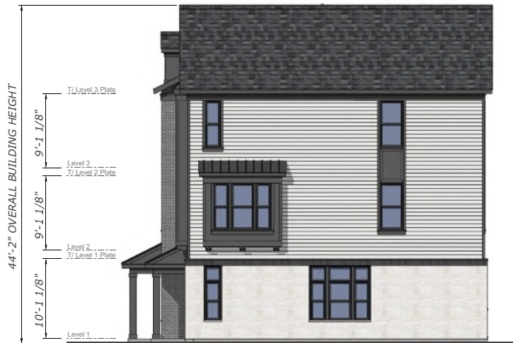
Unit 470 Side Elevation scale: 3/16" = 1'-0"
