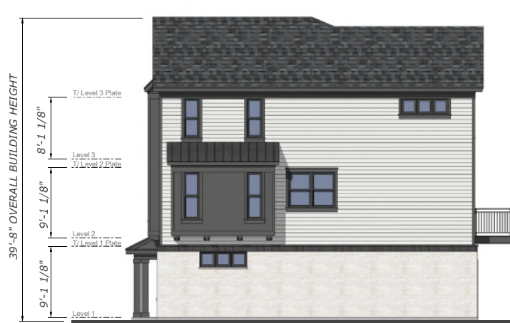
Unit 560 Side Elevation scale: 3/16" = 1'-0"
