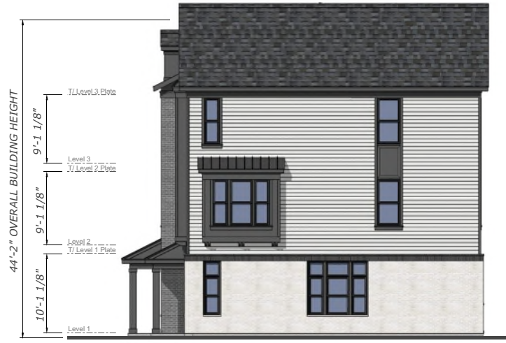
Side Elevation scale: 3/16" = 1'-0"
